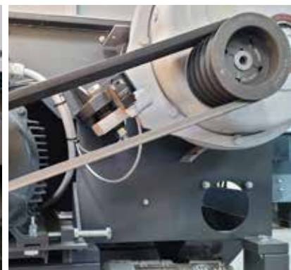
V-belt drive with gearbox limit switch
